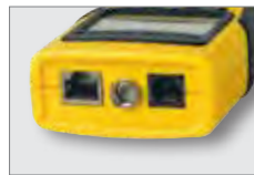
Top View: RJ45, RJ11/12 and F-connector ports
