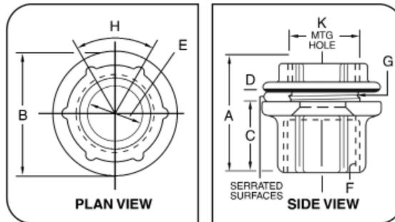
"D" dimension indicates maximum panel thickness hub will accommodate.
