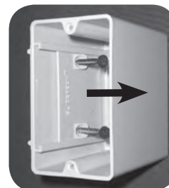
Slider plate retracted sets box in fully adjusted forward position for maximum wall substrate thickness of 1-3/8".
