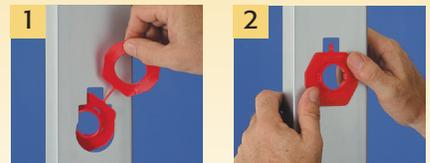
If a punched hole is required, the SB13 can be installed in a standard 1" trade size, round punched hole (1-3/8" diameter). Snap the bushing end into the hole.
