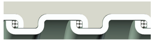
Square-Locked Design with cord packing 5/16" through 1-1/4"
