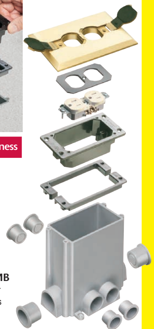
Supplied with 1/8", 1/4", 1/2" and 3/4" spacers to allow for increases in floor thickness; tile, wood, carpet, etc.
