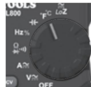
**!** Remove thermocouple before switching meter to other measurement functions.
