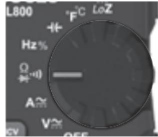
**NOTE:** When in a Resistance setting and the test leads are open (not connected across a resistor), or when a failed resistor is under test, the display will indicate O.L. This is normal.
