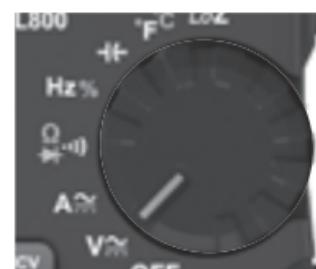
2. Apply test leads to the circuit to be tested to measure voltage. The meter will auto-range to display the measurement in the most appropriate range.
