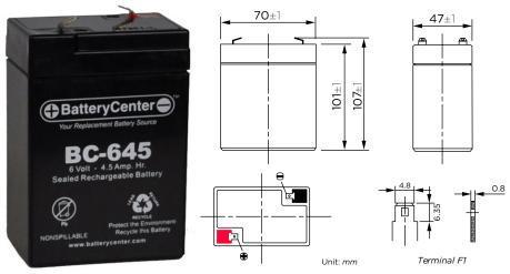
These rechargeable batteries are lead-lead dioxide systems. The dilute sulfuric acid electrolyte is absorbed by separators and thus immobilized. Should the battery be accidentally overcharged producing hydrogen and oxygen, special one-way valves allow the gases to escape thus avoiding excessive pressure build-up. Otherwise, the battery is completely sealed and is, therefore, maintenance-free, leak proof and usable in any position.
