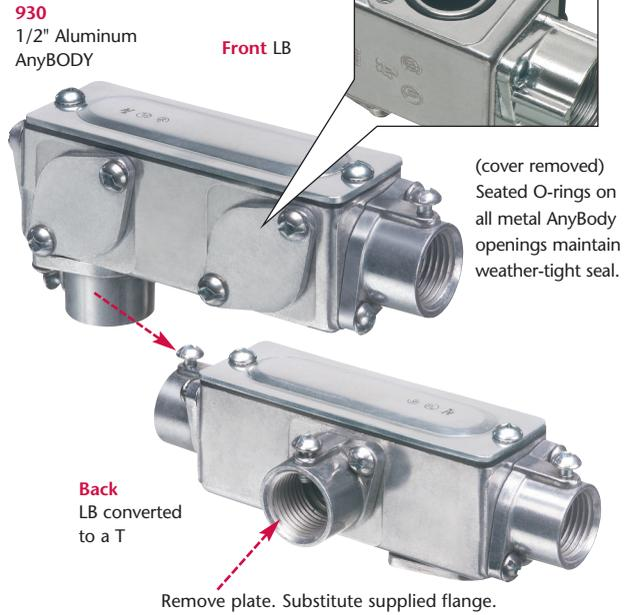
Meets NEC 2011 314.16 (c) (2) for Conduit Bodies with Splices, Taps or Devices.
