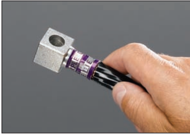
1. Crimp Multi-Tap connectors onto cables.
