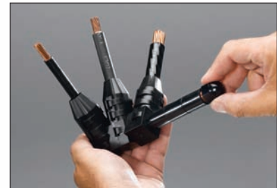
6. Reapply end nut and tighten.
