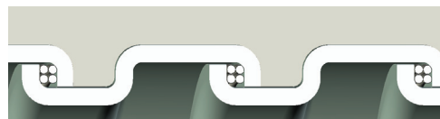
Square-Locked Design with cord packing 3/8" through 1-1/4"
