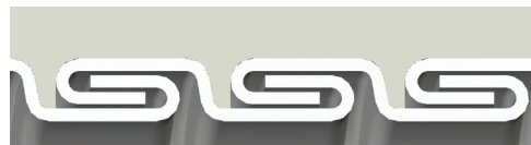
Interlocked Design 1-1/2" through 4"
