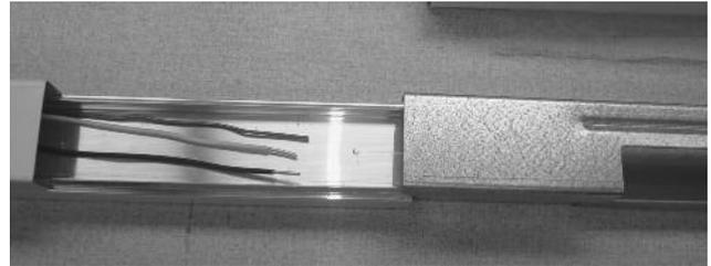
5. Tighten coupling hold-down screw.
