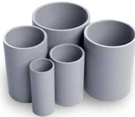
The Kraloy® molded repair couplings are specifically designed to facilitate the repair of existing conduit pipe. Their extended length and smooth internal diameter allow for easy installation and proper bonding of PVC cement over existing pipe to ensure a permanent and durable repair.
